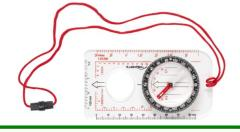
The needle in a compass is a magnet. A compass always points north-south on Earth.
